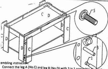
Connect the leg A (No.C) and leg B (No.D) with 3 in 1 screw (No.D) iden plug(No.3), tightening the 3 in 1 nut, and tightening the grub screw
